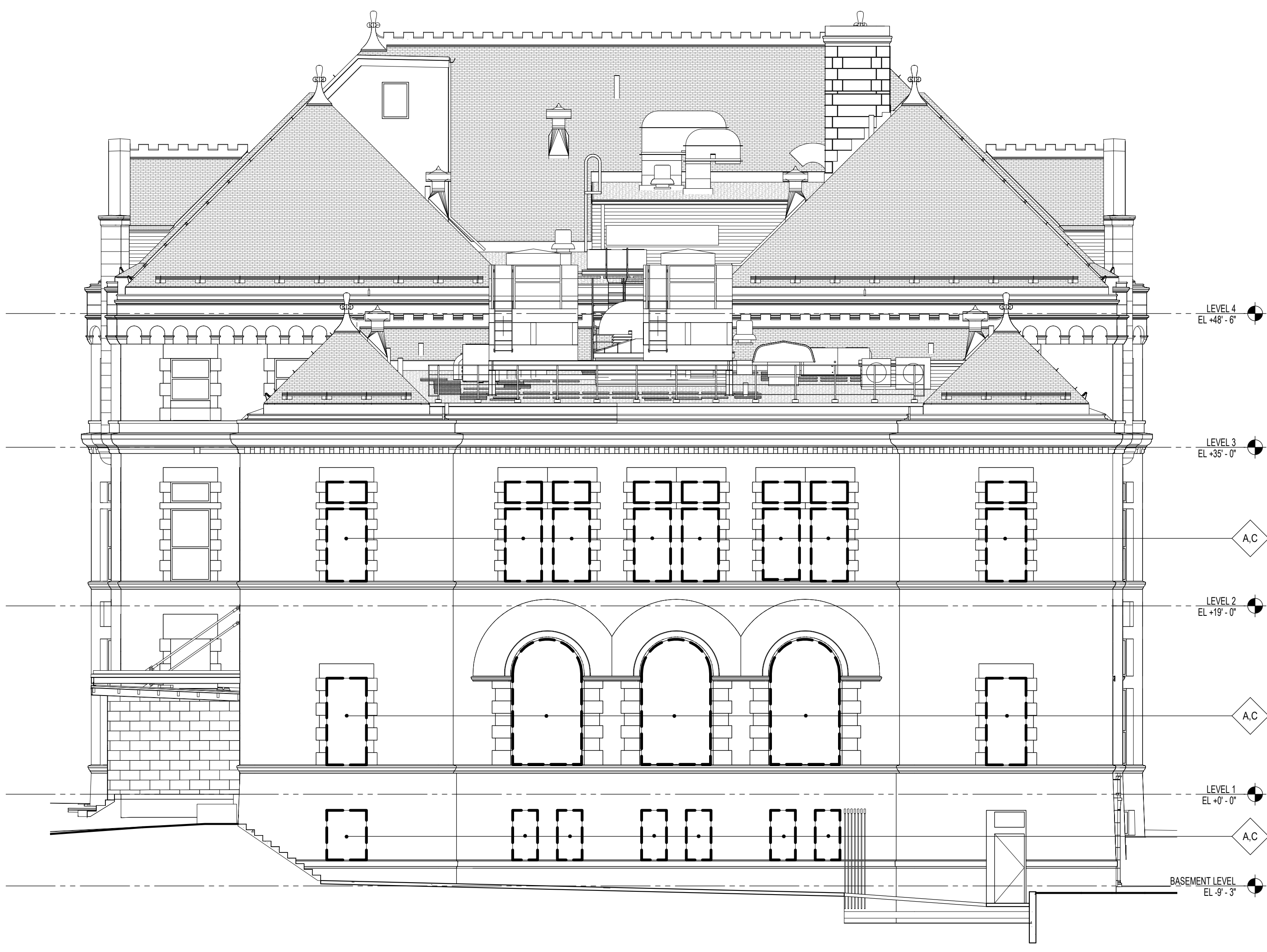
1 EAST ELEVATION - ADDITION SCALE: 1/8" = 1'-0"
