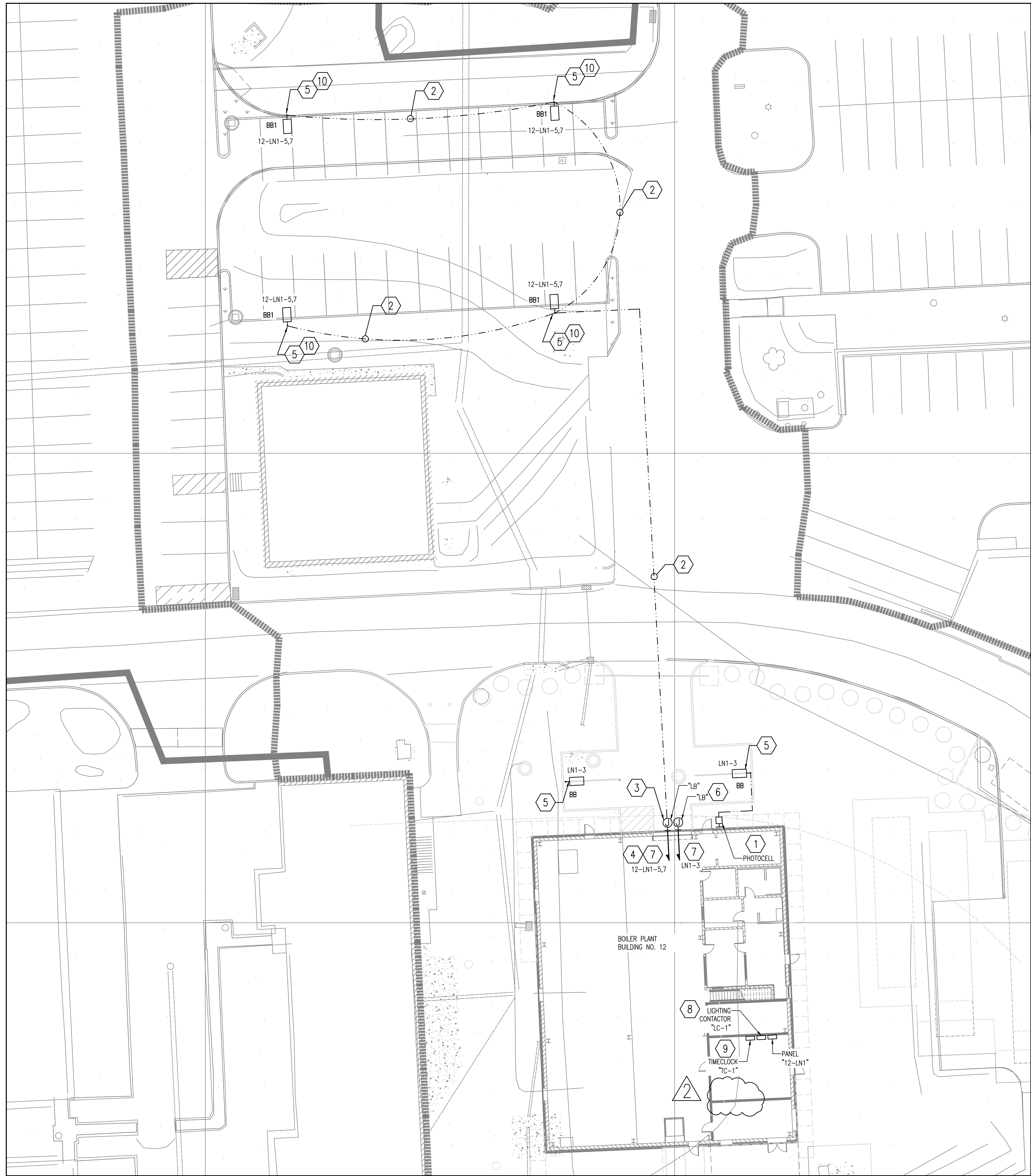
1 ELECTRICAL LIGHTING PLAN - PARKING LOT SCALE 1/8" = 1'-0"
