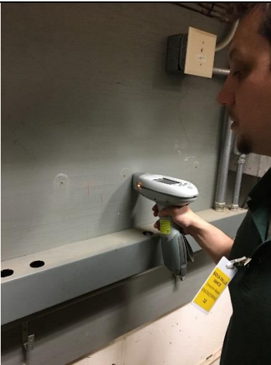
PHOTO 9 Gray Painted Wood Panel – Below Grade Mechanical Room <1mg/cm 2 lead
