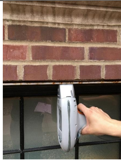
PHOTO 32 White Top Plate – Exterior Window 15 mg/cm 2 lead
