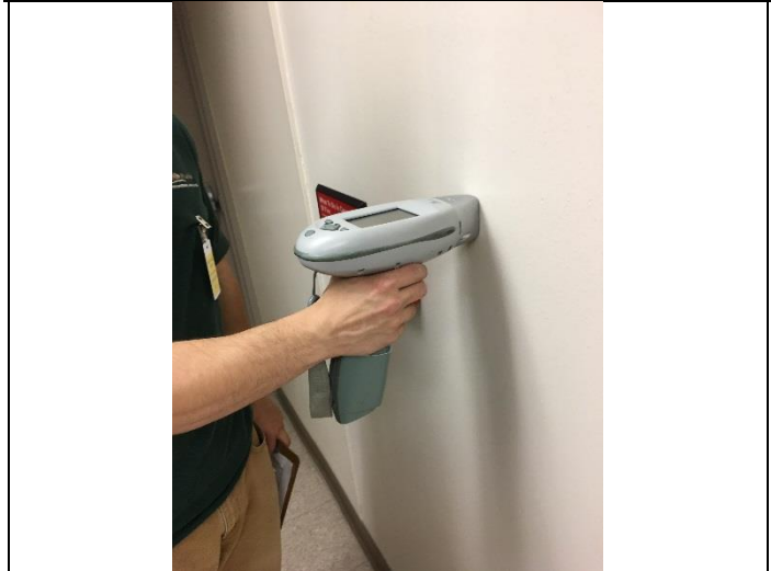
PHOTO 68 White Painted Sheetrock – West Wall <1mg/cm 2 lead
