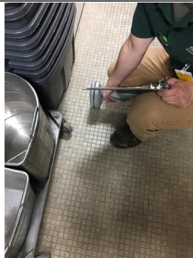
PHOTO 50 Beige Ceramic Tile Floor – D-17 <1mg/cm 2 lead
