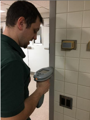
PHOTO 49 Beige Door Frame – D-17 <1mg/cm 2 lead
