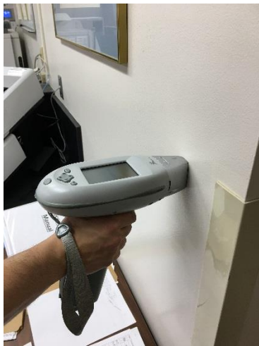
PHOTO 73 White Painted Sheetrock Wall - Lab <1mg/cm 2 lead
