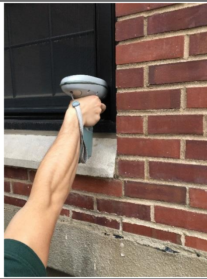
PHOTO 20 Black Window - Exterior <1mg/cm 2 lead
