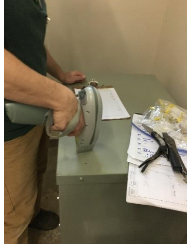
PHOTO 80 Transformer Box - D -20 <1mg/cm 2 lead
