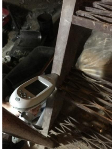
PHOTO 40 Brown Stairs to Tunnel 2.9 mg/cm 2 lead
