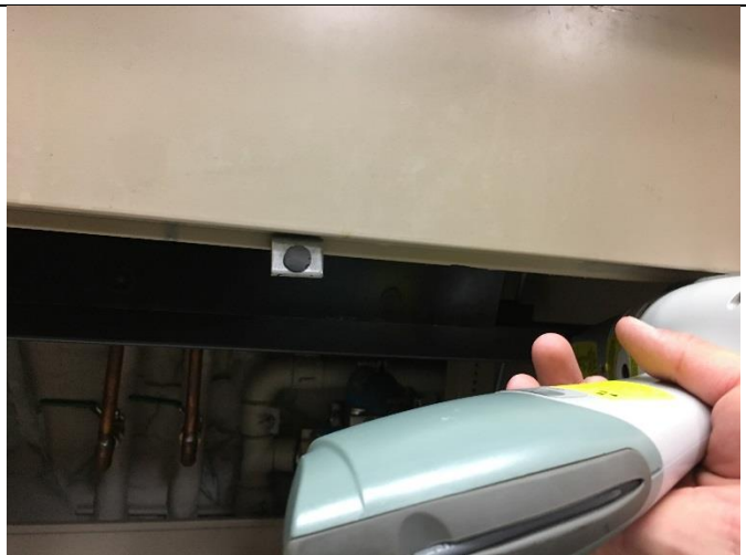
PHOTO 74 Black Metal surrounding sink basin <1mg/cm 2 lead
