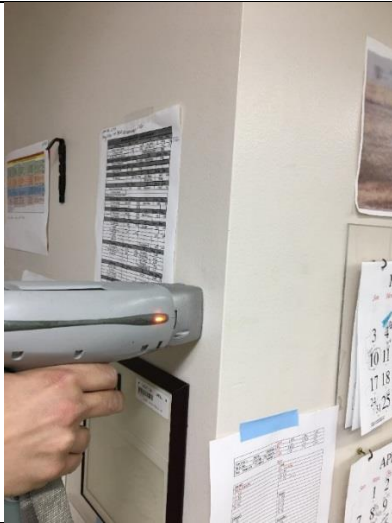
PHOTO 77 White Paint on Sheetrock - Lab <1mg/cm 2 lead
