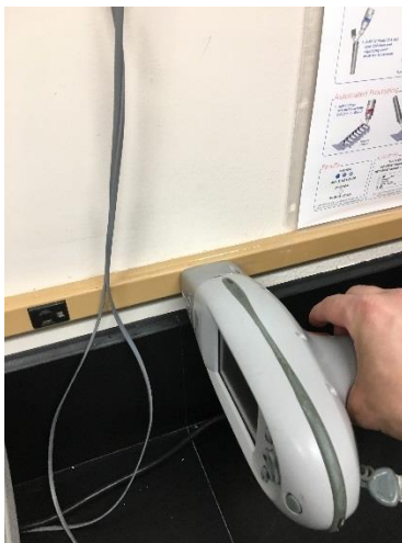
PHOTO 79 Metal Power Strip - Lab <1mg/cm 2 lead
