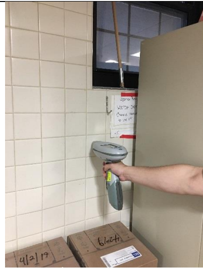
PHOTO 46 Cream Ceramic Tile – D-17 <1mg/cm 2 lead
