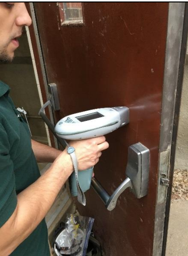
PHOTO 21 Red Mech. Room Door (Inside) <1mg/cm 2 lead
