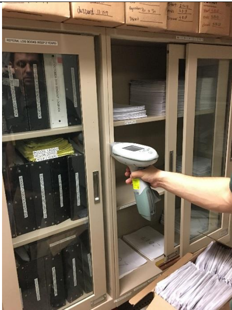
PHOTO 63 Beige Cabinet with Glass Room D-27 <1mg/cm 2 lead
