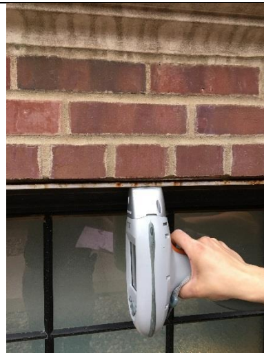
PHOTO 32 White Top Plate – Exterior Window 15 mg/cm 2 lead
