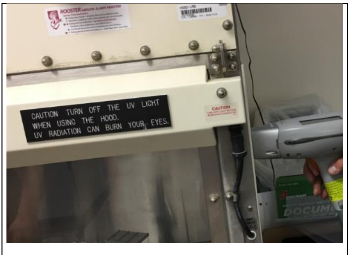
PHOTO 70 Cream Fume Hood – West Wall <1mg/cm 2 lead
