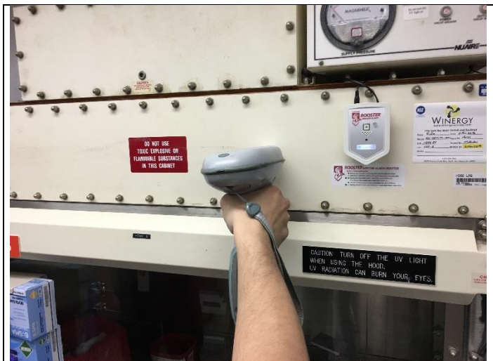
PHOTO 69 Cream Fume Hood – West Wall <1mg/cm 2 lead
