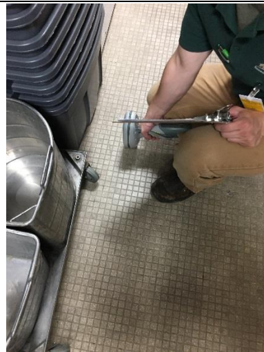
PHOTO 50 Beige Ceramic Tile Floor – D-17 <1mg/cm 2 lead
