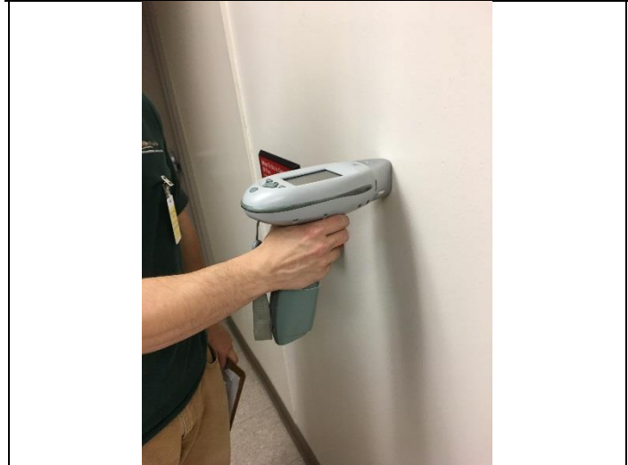
PHOTO 68 White Painted Sheetrock – West Wall <1mg/cm 2 lead
