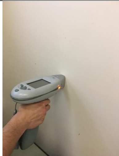
PHOTO 82 North Wall - D-20 <1mg/cm 2 lead
