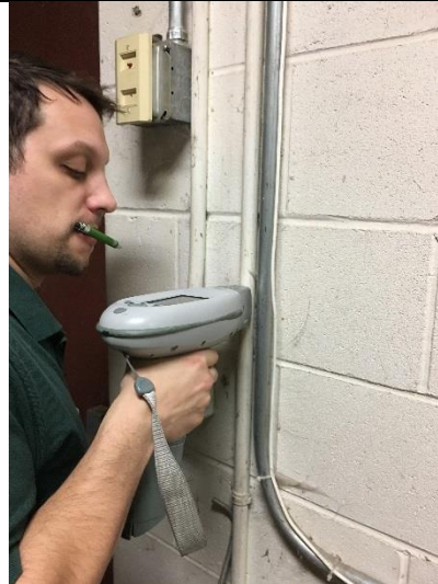
PHOTO 16 White Painted Conduit – Below Grade Mech. Room <math><1\text{mg}/\text{cm}^2\text{ lead}</math>
