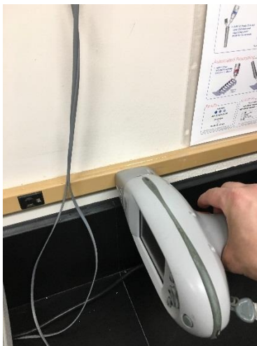
PHOTO 79 Metal Power Strip - Lab <1mg/cm 2 lead
