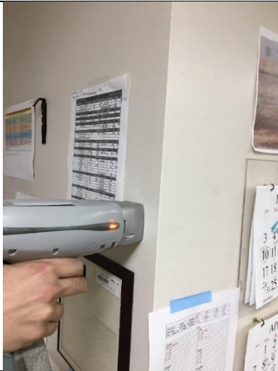
PHOTO 77 White Paint on Sheetrock - Lab <1mg/cm 2 lead
