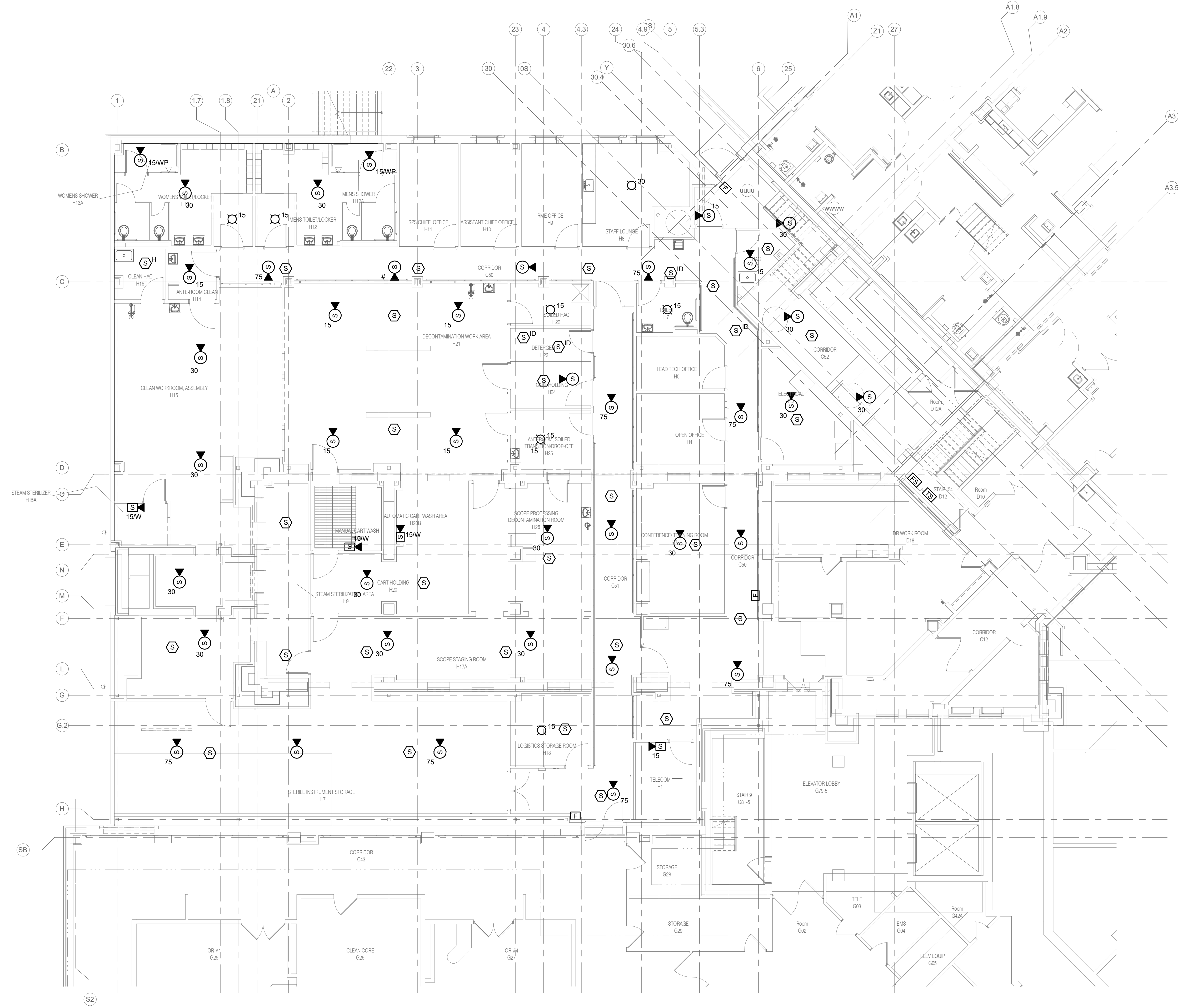
1 GROUND LEVEL FLOOR PLAN - FIRE ALARM 1/8" = 1'-0"
